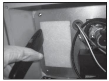
Figure 6.5 Cut and Remove Insulation
